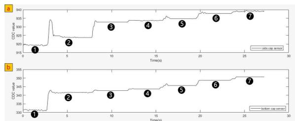
(Fig. 1.) Changes in capacitance value according to water volume
