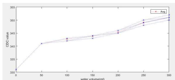
(Fig. 2.) Results of repeated tests on water volume measurement (Bottom sensor)
