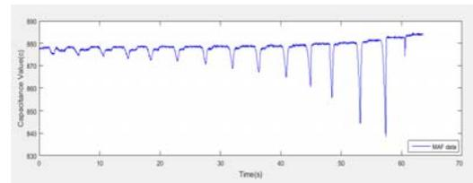
Fig. 5. MAF data of textile proximity sensor
