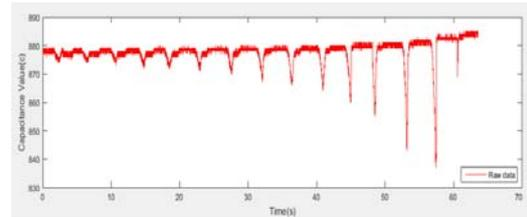
Fig. 4. Raw data of textile proximity sensor
