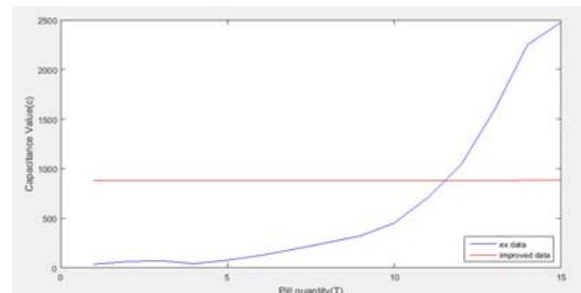
Fig. 6. Improved sensor data (red) and previous sensor data (blue) for quantity of pills
