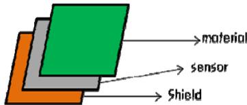
Fig. 1. Design of textile proximity sensor
