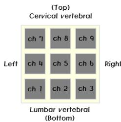
Figure 1. Backrest capacitive pressure sensor.
